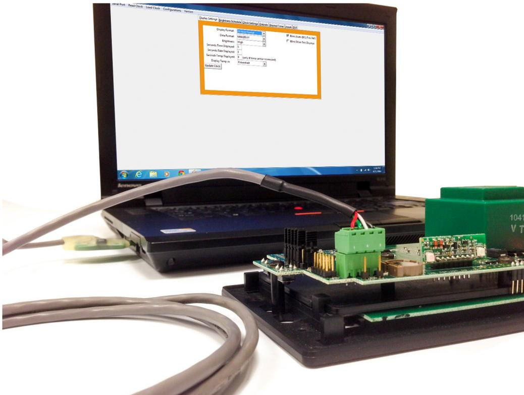
The optional USB cable will allow you to interface with Sapling's Configuration Software, which permits the user to access various settings in the digital clock. As shown in the above picture, one end of the USB cable will connect to a USB port on a PC and the other end will plug into the back of the digital clock. Detailed instructions on how to connect the USB Interface Cable and how to use the Configuration Software can be found in the Digital Clock Manual.
