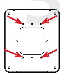
5) Use the positions of the marked holes to trace the location for your double gang box. It is VERY important that the holes on the gang box match the positions of the marked holes on the template. **Skip this if your clock is battery-powered.**
