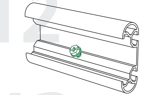
13) Mount the zone clock pole and attached housings to the bases by hanging the upper edge of the pole on the upper hooks of the base. Then, using the flathead screwdriver, turn the inner screw counterclockwise to activate the lower locking mechanism.
