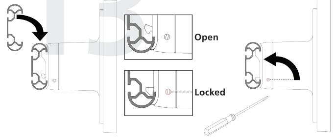
Test the pole to confirm that the locking mechanism has fully engaged. The pole should be able to slide side to side while attached to the base, but a user should not be able to lift the pole off of the base. **FAILURE TO FULLY ENGAGE THE LOCKING MECHANISM MAY RESULT IN USER INJURY.**
