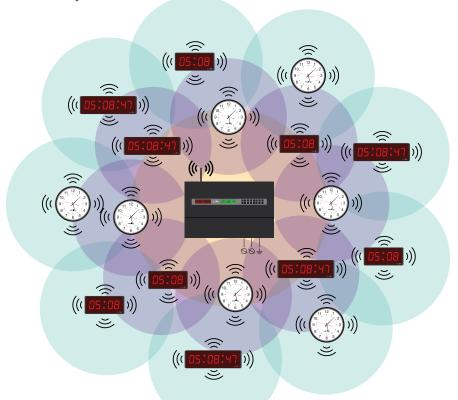
Sapling Wireless Clocks utilizing our patented built-in repeaters to create a mesh network
