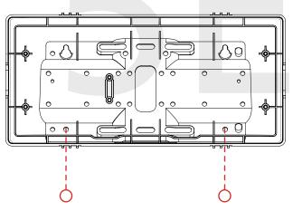
5F) Repeat step 5D, then pass another pair of #8 screws through the bottom holes and secure them in the remaining two wall anchors.
