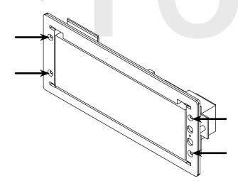
17) Use the 6-32x12 screws to attach the display board to the housing.
