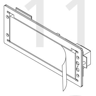
12) Place the filter over the display board. You should hear a snapping noise as the latches drop into place.
