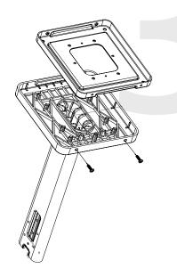
4) Attach the mounting plate to the gang box using only two of the four long, silver #6-32x1 screws. With the mounting plate as a guide, use the pencil to trace the locations of the four larger holes at the outer corners.
