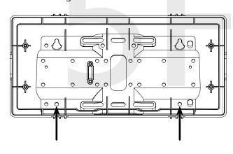
5G) Run power wires through the large hole in the back of the housing. Secure the wires by passing them through the wire clamp.
