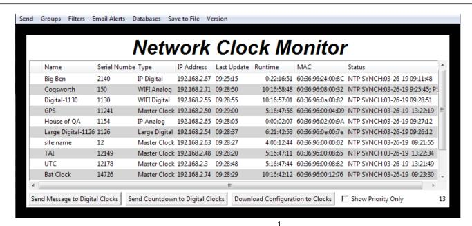
**1.Download Configuration to Clocks** - If a configuration file was created using "Upload and Save Configuration" on the Quick Access Menu, this option lets the user apply the configuration file to other clocks highlighted within the monitor. For more information, see the section of this manual labeled "Network Monitor Software - Quick Access Menu."
