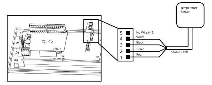
The Sensor Cable is 6 feet (1.83 meters) long, and so the sensor should be positioned within 6 feet of the clock. The cable is unshielded, 4 conductor, 22AWG (.33mm²). If longer than 6 feet is required, the wire would have to be terminated in an electrical box, and the longer wire would have to be provided by the customer.
