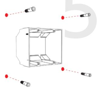
7) Thread any wiring through the mounting plate, and attach a grounding wire to the mounting plate using one of the larger centered holes and the #10-32x3/8 screw.
