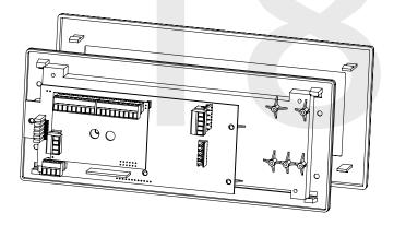
19) Place a housing frame onto each housing. You should hear a snapping noise as the latches drop into place.
