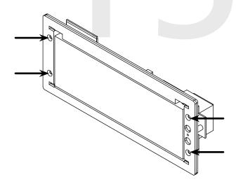
16) Use the M3.5-1.5x12 screws to attach a display board to each housing.
