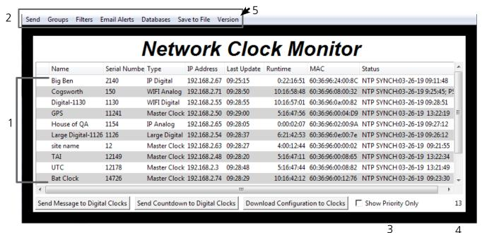
1. **Device List** - Displays all of the relevant IP devices that are active on the system subnet. The monitor screen displays the name of the clock, serial number, type of clock, IP address, last updated time, how long the clock has been running, and the status of the clock. Double clicking on a device in the device list will open the web interface for that device.
