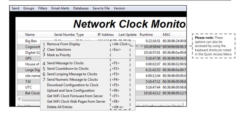
Using a right-handed mouse to right-click on any row in the Device List will open the Quick Access Menu.
