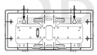
5C) Insert the wall anchors into the two holes, then place a #8 self-tapping screw into each wall anchor, leaving at least a 1/8" gap between the top of the screw and the wall.
