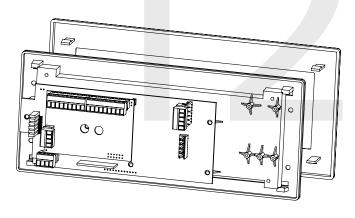
13) Place the housing frame onto the housing. You should hear a snapping noise as the latches drop into place.
