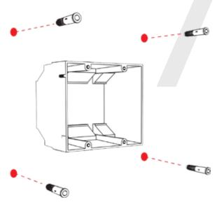
9) Thread any wiring through the mounting plate, and attach a grounding wire to the mounting plate using one of the larger centered holes and the #10-32x3/8 screw.
