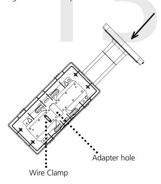
12) Insert the four #8-32x7/16 screws through the internal-tooth washers, then through the adapter, and finally into the pole. Use a screwdriver to tighten the screws so that the adapter does not move.
