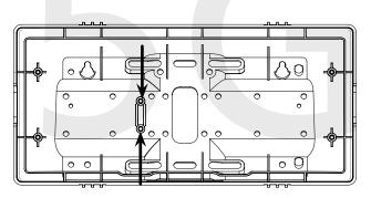
6) Perform step 5G, then attach the housing to the gang box using the #6-32x1 screws.
