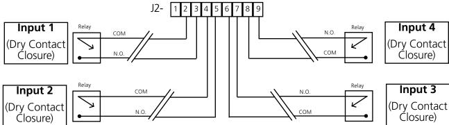
Use a dry contact closure between any of the two lines shown above to activate one of the numbered user inputs. This input is a *dry contact closure*, which means that **the user should not be providing external power on either of the lines leading from the relay to the clock.** The dry contact closure only needs to complete the circuit when activated, and can be a simple switch or button.
