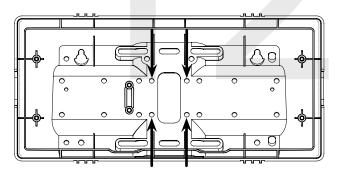
14) Detach the filter from the clock display board by pressing inward on the red tabs.
