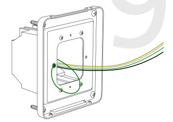
8) Reattach the mounting plate, this time using all four long, silver #6-32x1 screws, then insert the four #8 screws through the mounting plate and into the anchors.
