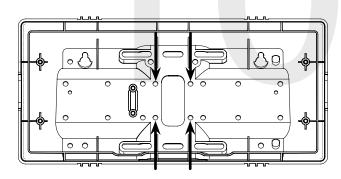
11) Attach adapters to each other using adapter tab screws, two on each side.
