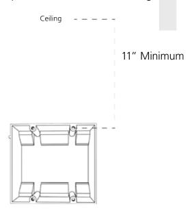
2) Run power and accessory wiring to the gang box.
