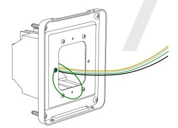
6) Reattach the mounting plate, this time using all four long, silver #6-32x1 screws, then insert the four #8 screws through the mounting plate and into the anchors.
