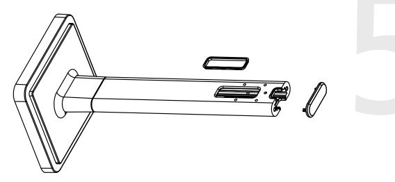
6) Attach the flag-mount end cap to the pole. Confirm that the covering flap is attached to the side where the plastic ring was removed.
