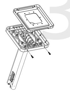
4) Attach the mounting plate to the gang box using only two of the four long, silver #6-32x1 screws. With the mounting plate as a guide, use the pencil to trace the locations of the four larger holes at the outer corners.
