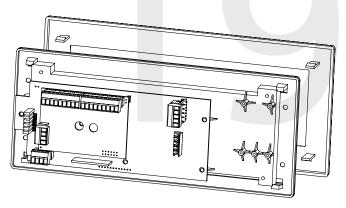
20) Place the housing frame onto the housing. You should hear a snapping noise as the latches drop into place.
