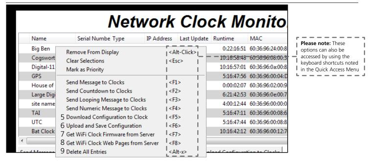
Using a right-handed mouse to right-click on any row in the Device List will open the Quick Access Menu.
