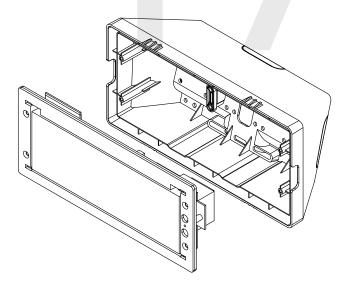
18) Remove the plastic cover from the display board.
