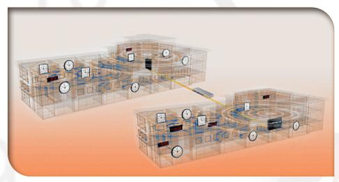
What type of information does the clock tell the master clock? The clocks communicate their battery life, signal strength and even their mechanical status. The master clock then takes the information and stores it, so it can be shown on its built-in web browser or through its e-mail notification system. All of this is capable while still preserving
