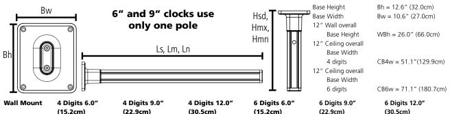
**Std Pole Length:** Ls = 37.1'' (94.2cm) Ls = 47.8'' (121.4cm) Ls = 58.4'' (148.3cm) Ls = 47.6'' (120.8cm) Ls = 63.0'' (160.0cm) Ls = 78.4'' (199.1cm) Max Pole Length: Lm = 45.4" (115.2cm) Lm = 56.1" (142.4cm) Lm = 66.7" (169.4cm) Lm = 55.8" (141.8cm) Lm = 71.2" (181.9cm) Lm = 86.7" (220.1cm) Min Pole Length: Ln = 33.4" (84.7cm) Ln = 44.1" (111.9cm) Ln = 54.7" (138.9cm) Ln = 43.8" (111.3cm) Ln = 59.2" (150.4cm) Ln = 74.6" (189.6cm)
