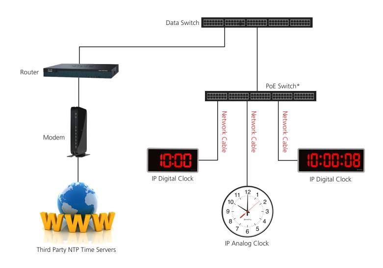
\*PoE Switch is required for IP Analog & IP Digital Clocks
