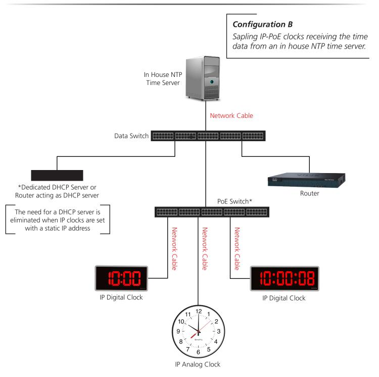
\*PoE Switch is required for IP Analog & IP Digital Clocks
