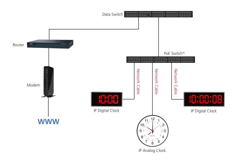
\*PoE Switch is required for IP Analog & IP Digital Clocks
