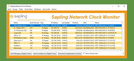
Sapling Network Clock Monitoring Software allows the user to oversee their whole system from one
