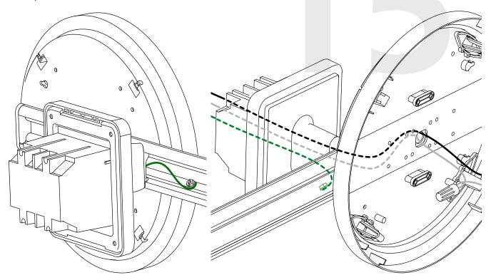
16) Run wiring or IP cables to the remaining clocks. Thread wiring through the white cable anchors where applicable (this may have already been done for you, if it is a wire-powered system).
