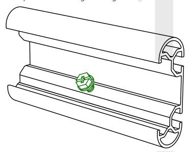
13) Mount the zone clock pole and attached housings to the bases by hanging the upper edge of the pole on the upper hooks of the base. Then, using the flathead screwdriver, turn the inner screw counterclockwise to activate the lower locking mechanism.
