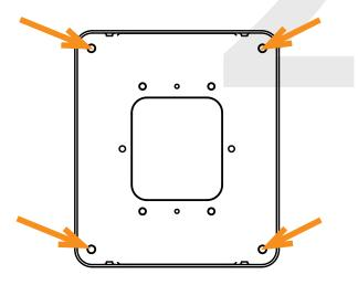
3) **Skip this step if your clock is battery-powered.** Use a pencil to poke through the template and find the position of each inner hole. Mark each position on the wall.
