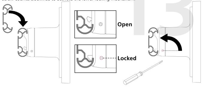
Test the pole to confirm that the locking mechanism has fully engaged. The pole should be able to slide side to side while attached to the base, but a user should not be able to lift the pole off of the base. **FAILURE TO FULLY ENGAGE THE LOCKING MECHANISM MAY RESULT IN INJURY.**
