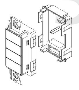
2) Remove the face of the Elapsed Timer by unscrewing the two screws on the front cover.
