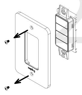
4) There will be a pair of holes above and below the buttons. Align the holes closest to the buttons with the connection holes on the gang box. Use screws to attach the control panel to the gang box. Do not use the outer holes as they are for the front panel screws. Remove the circuit board and set it aside.
