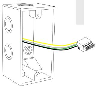
3) Attach the control panel to the power and communications cable by inserting the green connector into the port.
