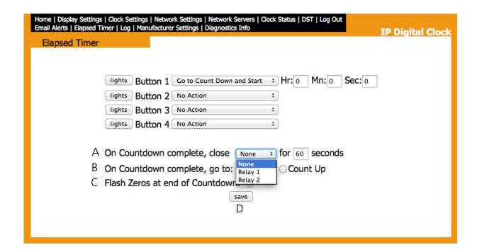
**A.** When a user schedules a countdown, they may also command a relay to close after a countdown is complete (if using a 3300 Series Digital Clock). This is configured through the configuration window or web interface. Listed below are the options for this function:
