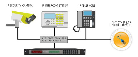
Sapling offers an NTP Master Clock Server that may provide the time data to IP devices in the facility such as:
