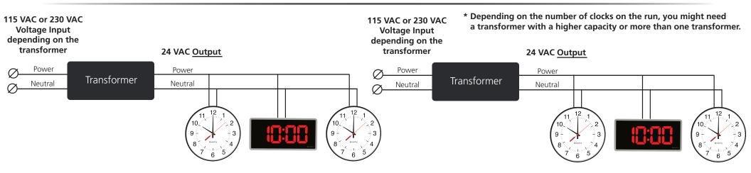
In a Sapling Wired, Wireless, or Wi-Fi Clock System, Sapling offers the option of analog or digital clocks powered at 24 VAC. In this low voltage application, a transformer will reduce local power to 24 VAC and provide 24 VAC to the clocks. The clocks will be wired to the transformer in a parallel (T-tap) connection, and therefore an issue with one clock will not affect any other clocks in the system.
