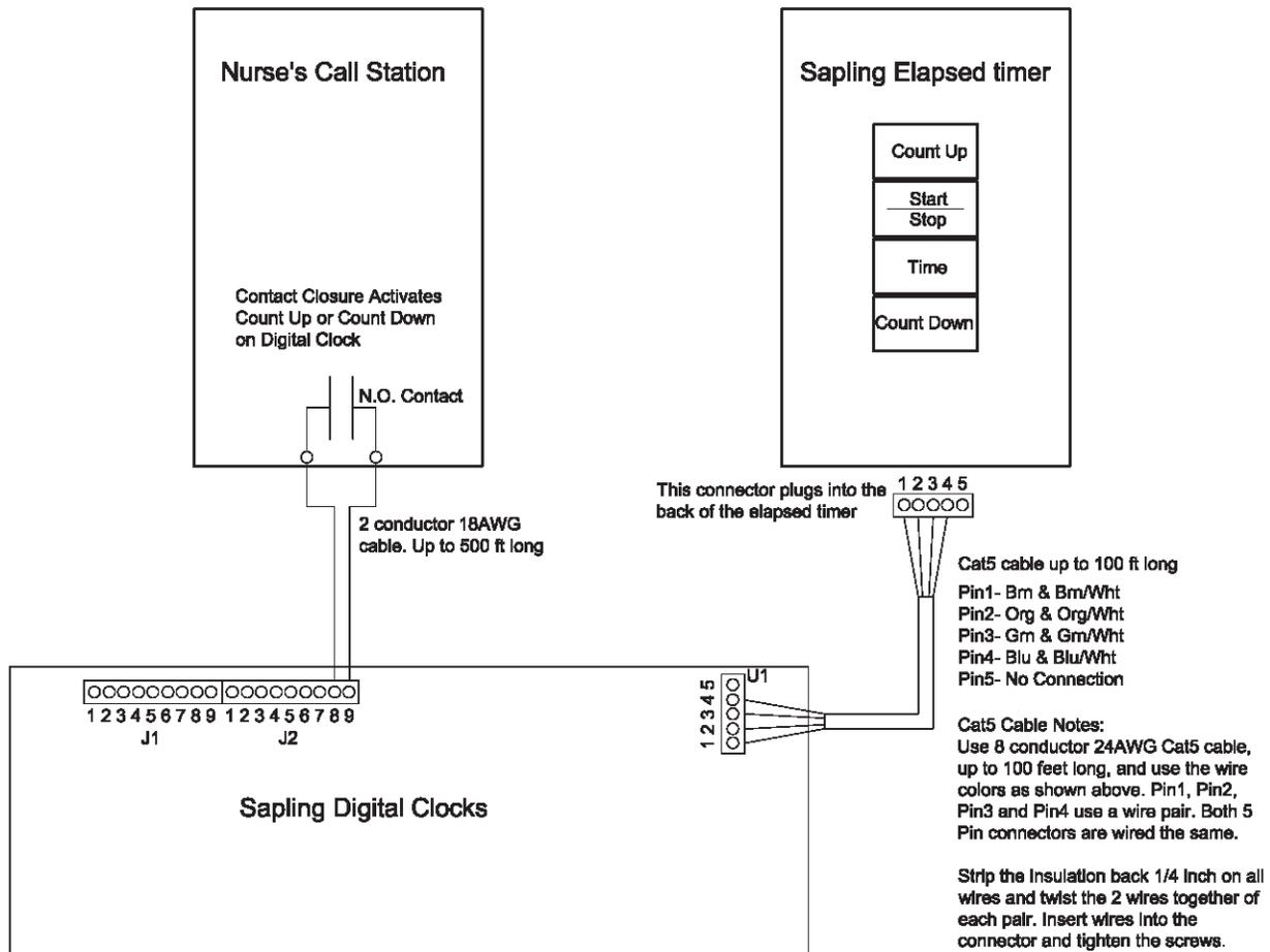
Sapling's 3300 Series digital clock model is capable of interfacing with both an Elapsed Timer Control Panel for manual activation of a count up (or count down), as well as a nurse call system which will trigger the count up automatically.
