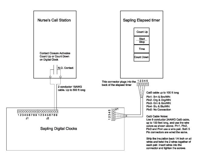
Sapling's 3300 Series digital clock model is capable of interfacing with both an Elapsed Timer Control Panel for manual activation of a count-up (or countdown), as well as a nurse call system, which will trigger the count-up automatically.
