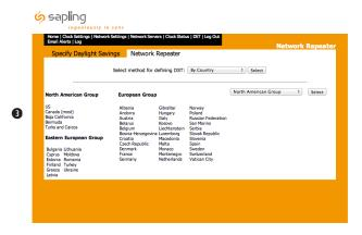
**Selecting DST by Country Option** - This Daylight Saving Time option is used when the time is to be changed time based on what country its located in. Select the pre-defined group that best fits which DST setting is desired.
